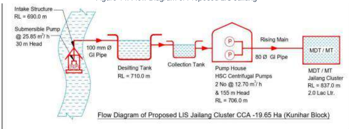
Figure 14: Flow Diagram of Proposed LIS Jailang
